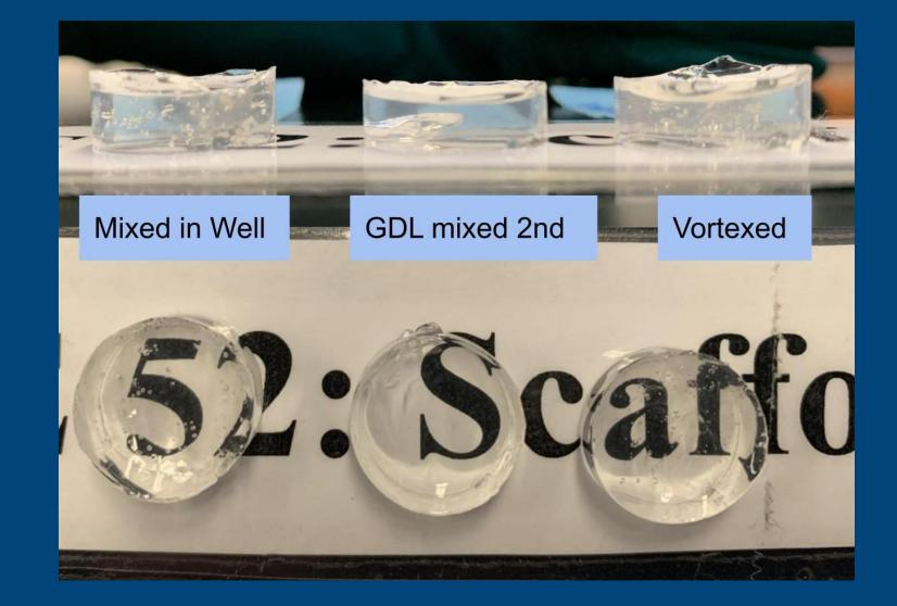
3% alginate solution with 50 mM CaCO<sub>3</sub> and 100 mM GDL. Different mixing methods and order of mixing were tested to find optimum clarity in samples with minimal bubbles. Mixing GDL in second helped reduce the number of bubbles in the gel, thus resulting in a more transparent sample.
