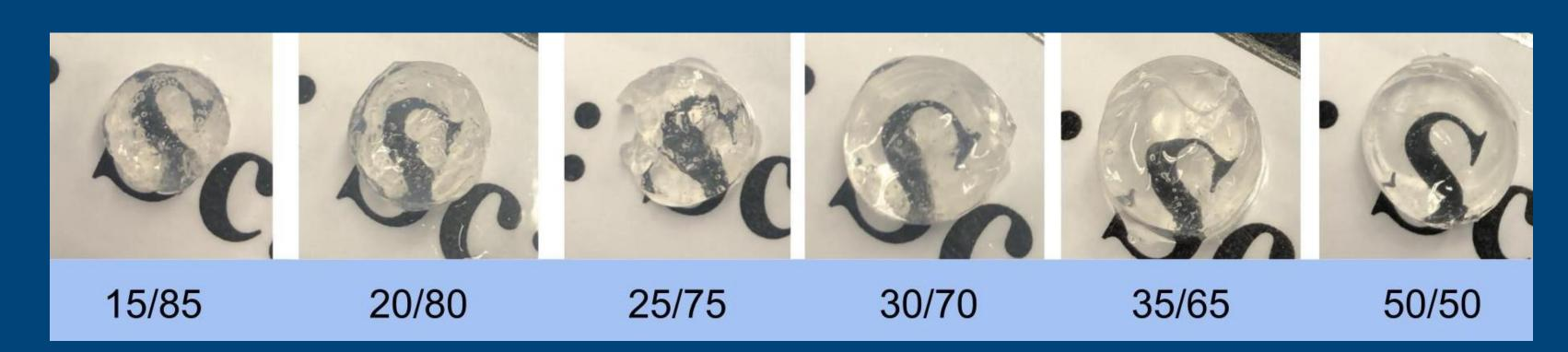
Different ratios of sodium alginate to CaCO<sub>3</sub>/GDL concentrations were tested for maximum transparency and minimal bubble formation in the gel, leading to the determination that a 50/50 volumetric ratio was optimal.
