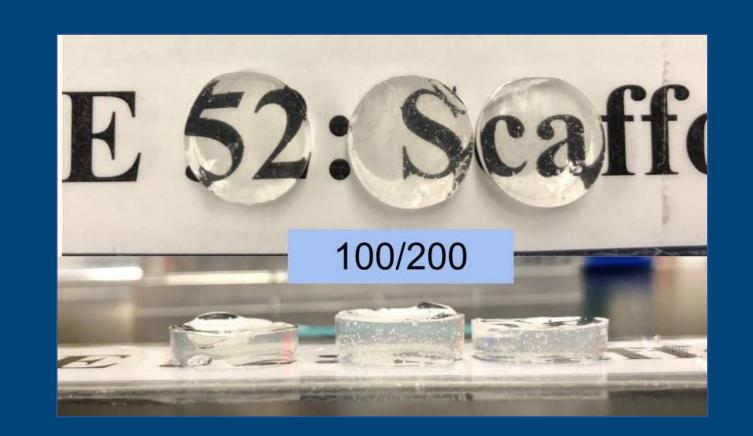
Different CaCO<sub>3</sub> and GDL concentrations were tested for their effect on the structural integrity of the gels. Higher concentrations of CaCO<sub>3</sub> yielded firmer gels with higher Young's moduli, due to higher cross-linking density. This ratio also yielded gels that better maintained mold morphology.
